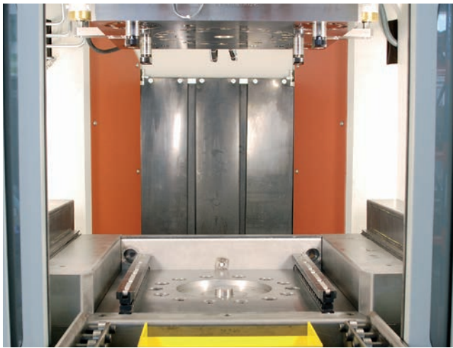
The enlarged tool space of the XFT 2500speed
