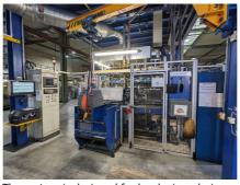
The system is designed for hardening, drying and oiling cam tubes.
