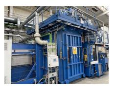
Isothermal forging is a type of forging process that involves shaping a material while maintaining its temperature at a constant level throughout the forging process.
