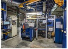
The system is designed for hardening, drying and oiling cam tubes.
